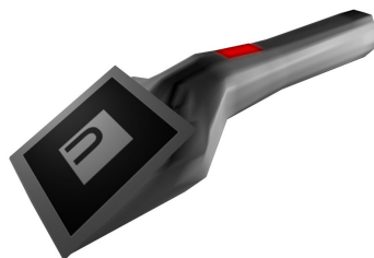
Figure 5: Gripper with button (red) and a distinct marker.
