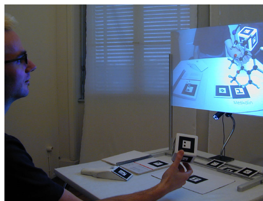
Figure 13: Viewing a predefined (saturated) molecule in the browser mode while using the cube to rotate the model.
